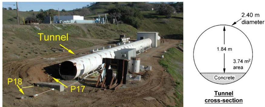
Fig. 7. Tube modeling a tunnel and the cross-section.
