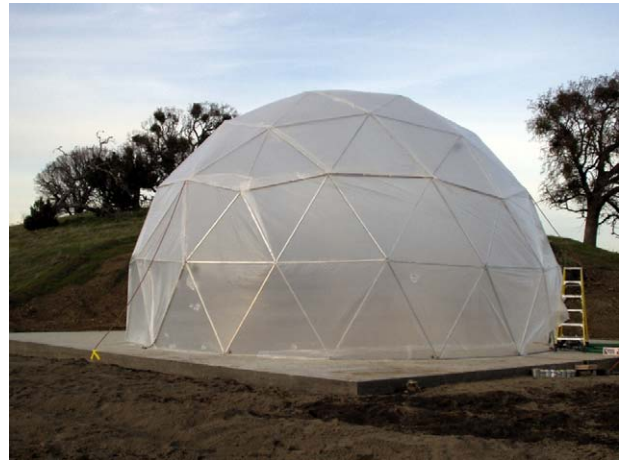
Fig. 3. Tent (300-m 3 ) for homogeneous concentration gas mixture (9.7 m (diameter of bottom) × 5.7 m (height)).
